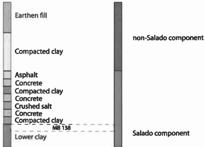
Figure 2: Representation of the baseline shaft seal model contrasted with the proposed simplified model.
