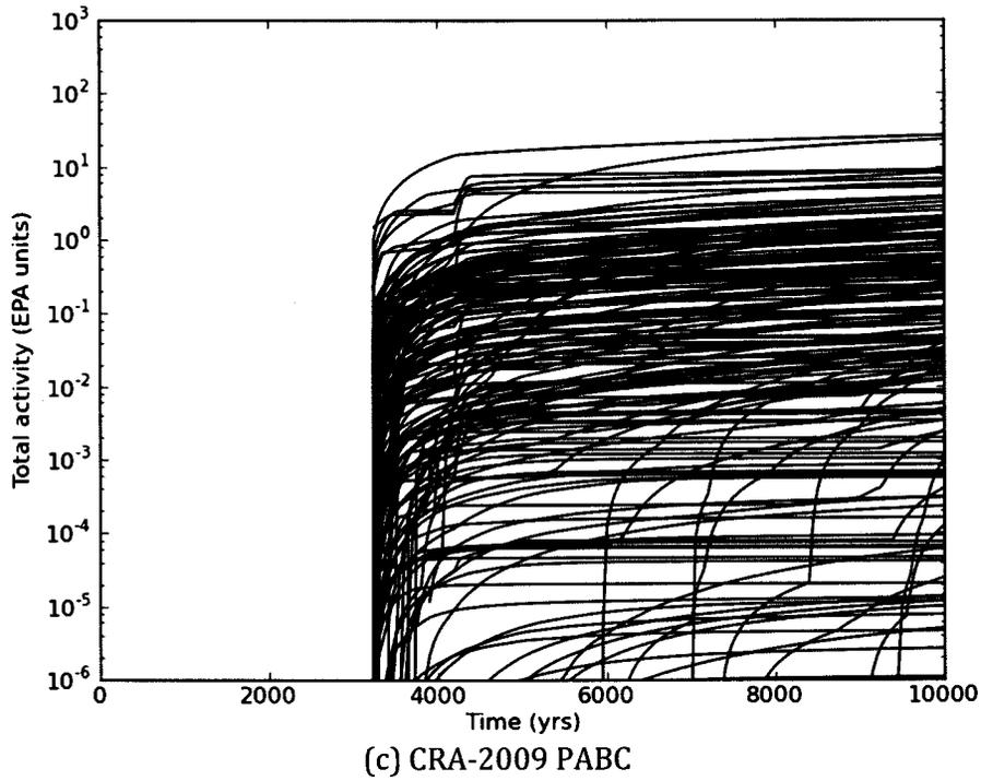
**Figure 15(c)** Cumulative total releases to the Culebra for an E1 intrusion at 3000 years in the (a) CRA-2014 PA, (b) CRA-2014 BL, and (c) CRA-2009 PABC.
