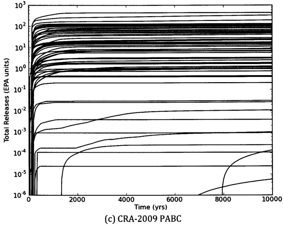
**Figure 26(c)** Cumulative total releases to the Culebra for an E2-E1 intrusion at 100 years in the (a) CRA-2014 PA, (b) CRA-2014 BL, and (c) CRA-2009 PABC.
