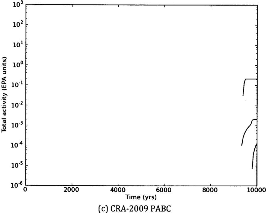
**Figure 25(c)** Cumulative total releases to the Culebra for an E2 intrusion at 9000 years in the (a) CRA-2014 PA, (b) CRA-2014 BL, and (c) CRA-2009 PABC.
