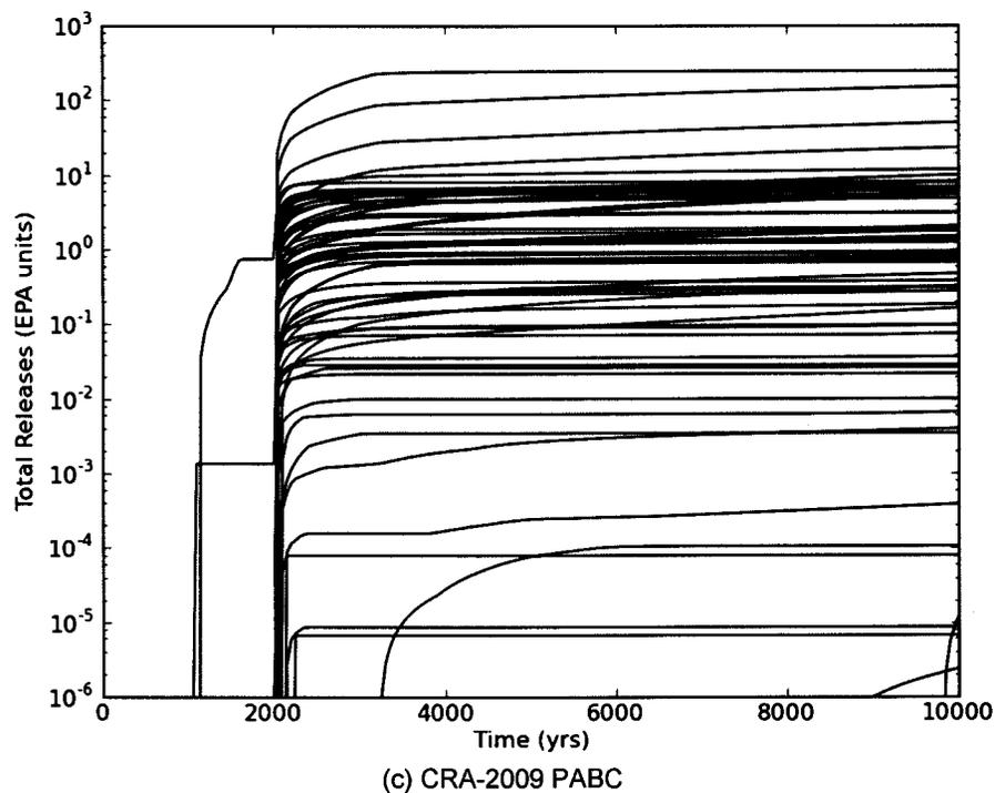
**Figure 9(c)** Total releases to the Culebra for Replicate 1, Scenario S6-BF in the (a) CRA-2014 PA, (b) CRA-2014 BL, and (c) CRA-2009 PABC.
