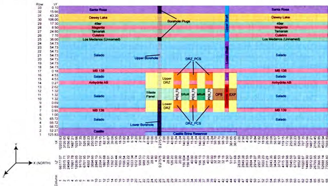
**Figure 1** Computational grid used for Salado Flow and transport calculations.
