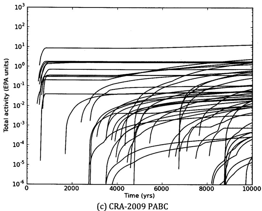
**Figure 19(c)** Cumulative total releases to the Culebra for an E2 intrusion at 100 years in the (a) CRA-2014 PA, (b) CRA-2014 BL, and (c) CRA-2009 PABC.
