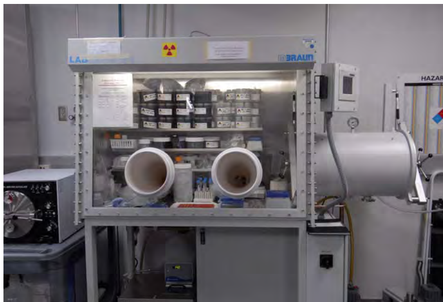
Figure 4-7. Mbraun re-circulating glovebox used for the ACRSP plutonium experiments
