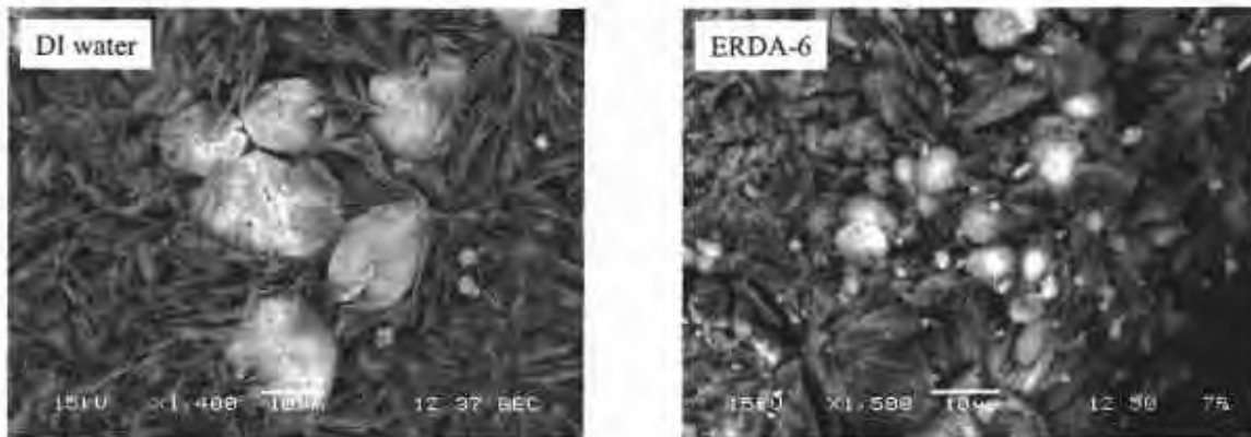
Figure 3. SEM images of Ca-carbonates (white) surrounded by brucite (gray) after 141 days.
