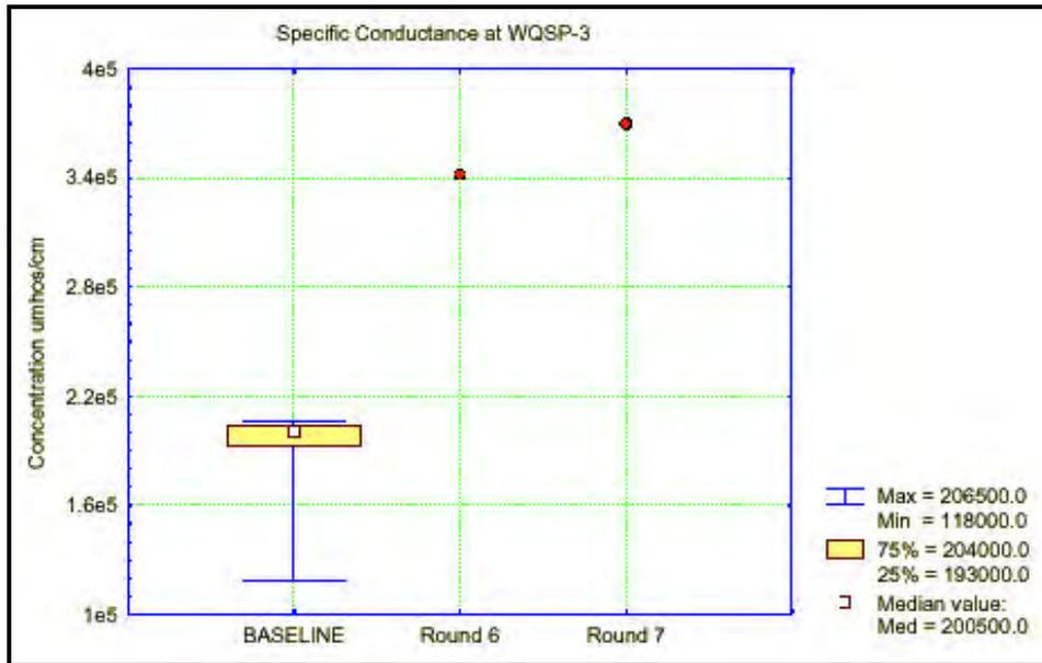
Figure 7.23 - Time Trend Plot for Specific Conductance at WQSP-3
