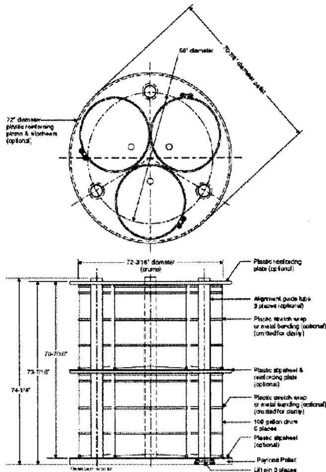
Figure 2. Six 100-Gallon Drum Payload Assembly Configuration (DOE 2000, Figure 2.1-7)
