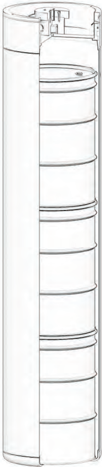
Figure 2. Removable Lid RH Canister with three 55-Gallon Drum Payload
