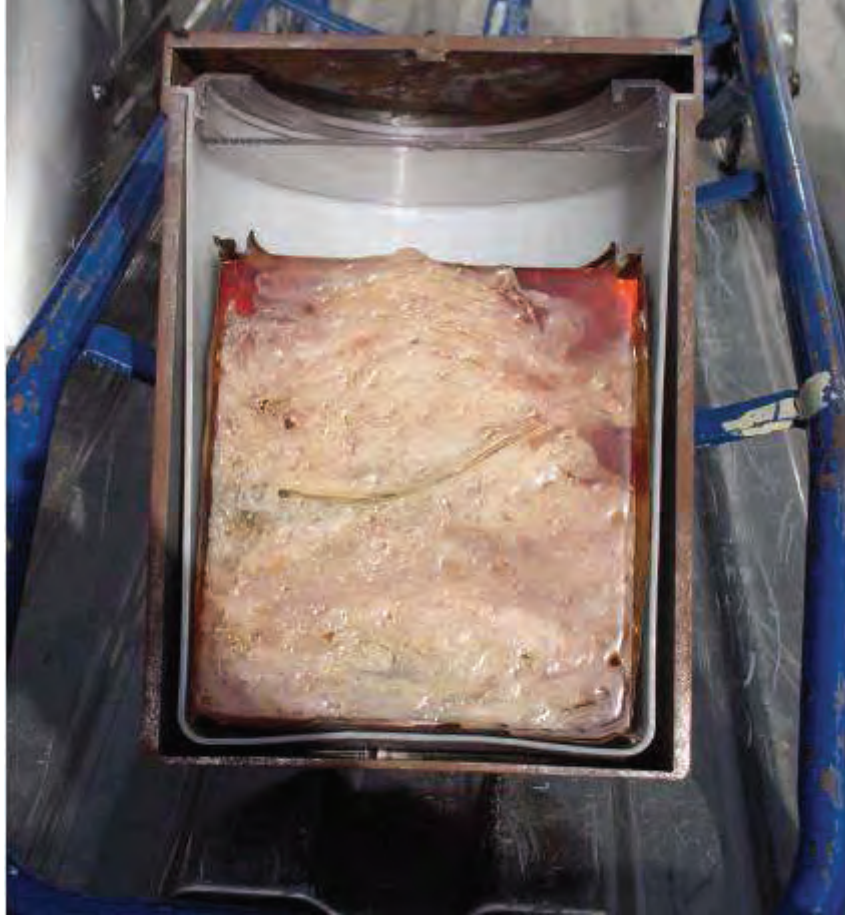
Figure 1. Cut-away View of a Paint Can Inside an Alpha Can Inside a 1/2-Gallon Steel Can that Has Been Welded Shut
