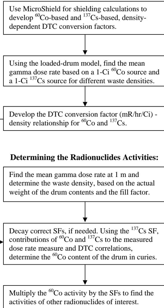
**Figure 6. Flow Diagram for the Radiological Characterization of Waste Stream SR-BCLDP.004.003**
