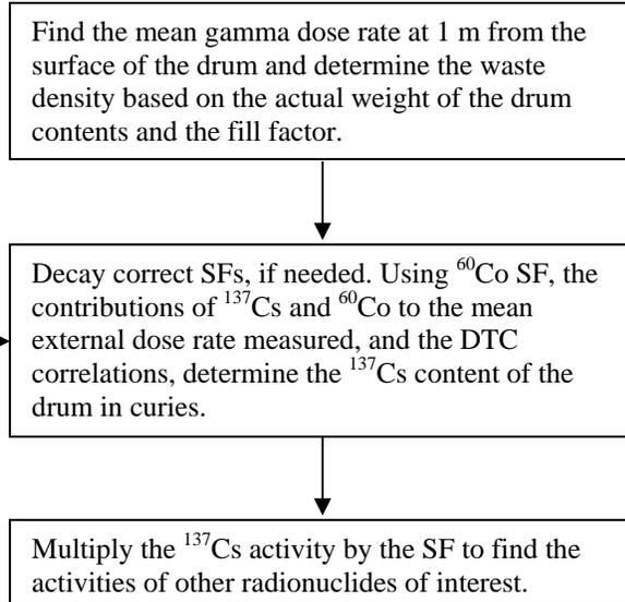
**Figure 4. Flow Diagram for the Radiological Characterization of Waste Stream SR-BCLDP.003**
