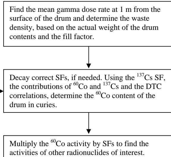
**Figure 5. Flow Diagram for the Radiological Characterization of Waste Stream SR-BCLDP.004.002**
