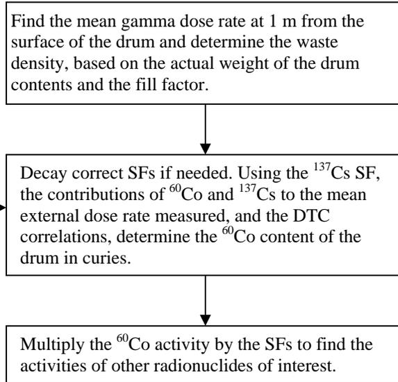
**Figure 2. Flow Diagram for the Radiological Characterization of Waste Stream SR-BCLDP.001.002**
