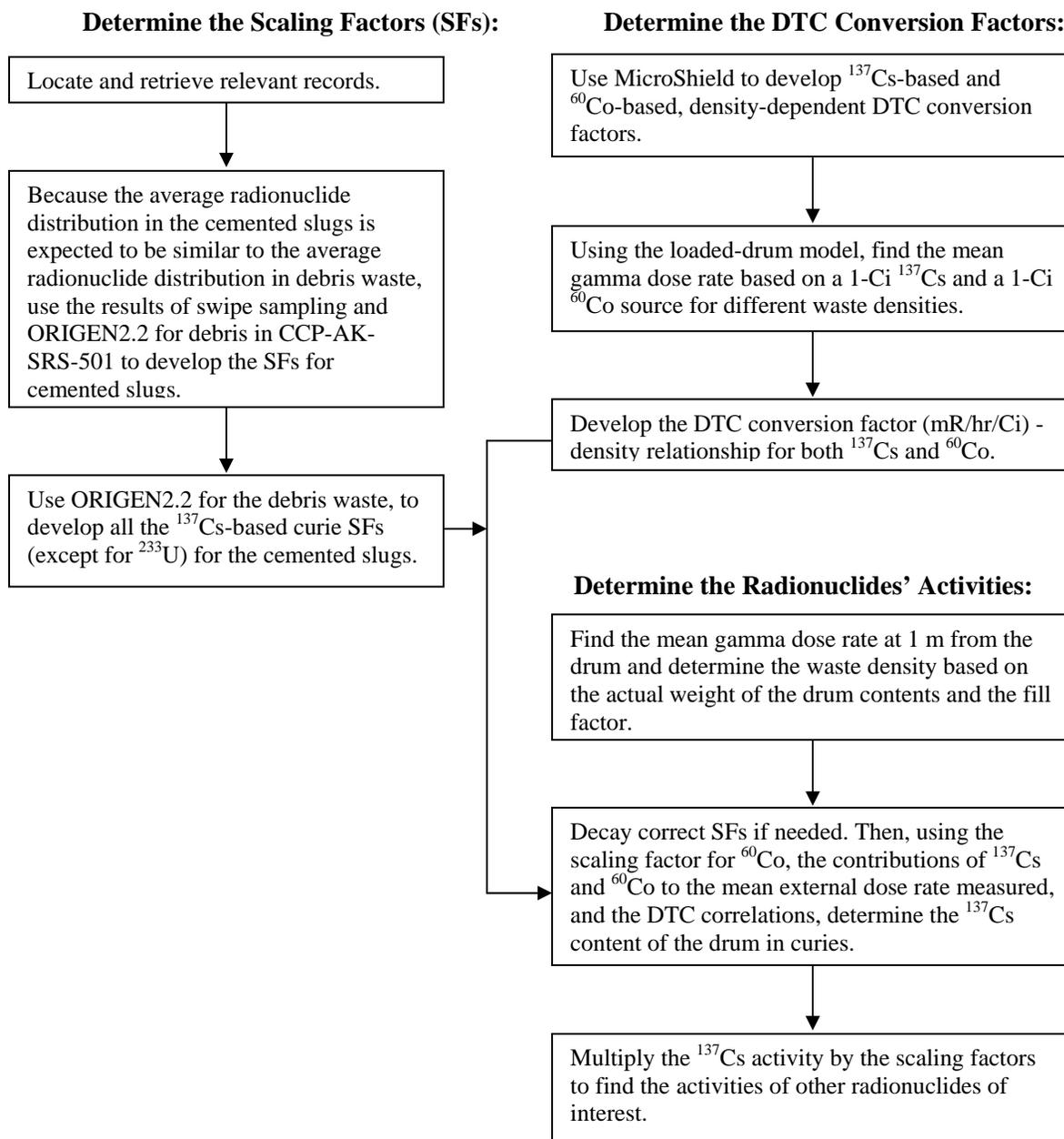
**Figure 3. Flow Diagram for Waste Stream SR-RL-BCLDP.002**
