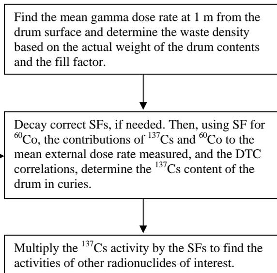
**Figure 1. Flow Diagram for the Radiological Characterization of Waste Stream SR-BCLDP.001.001**
