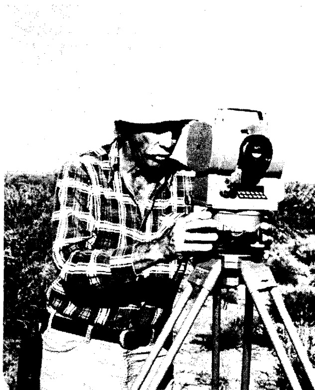
Figure 1.3.1-2. Surveyor with Hewlett-Packard model 3820A laser rangefinder/theodolite
