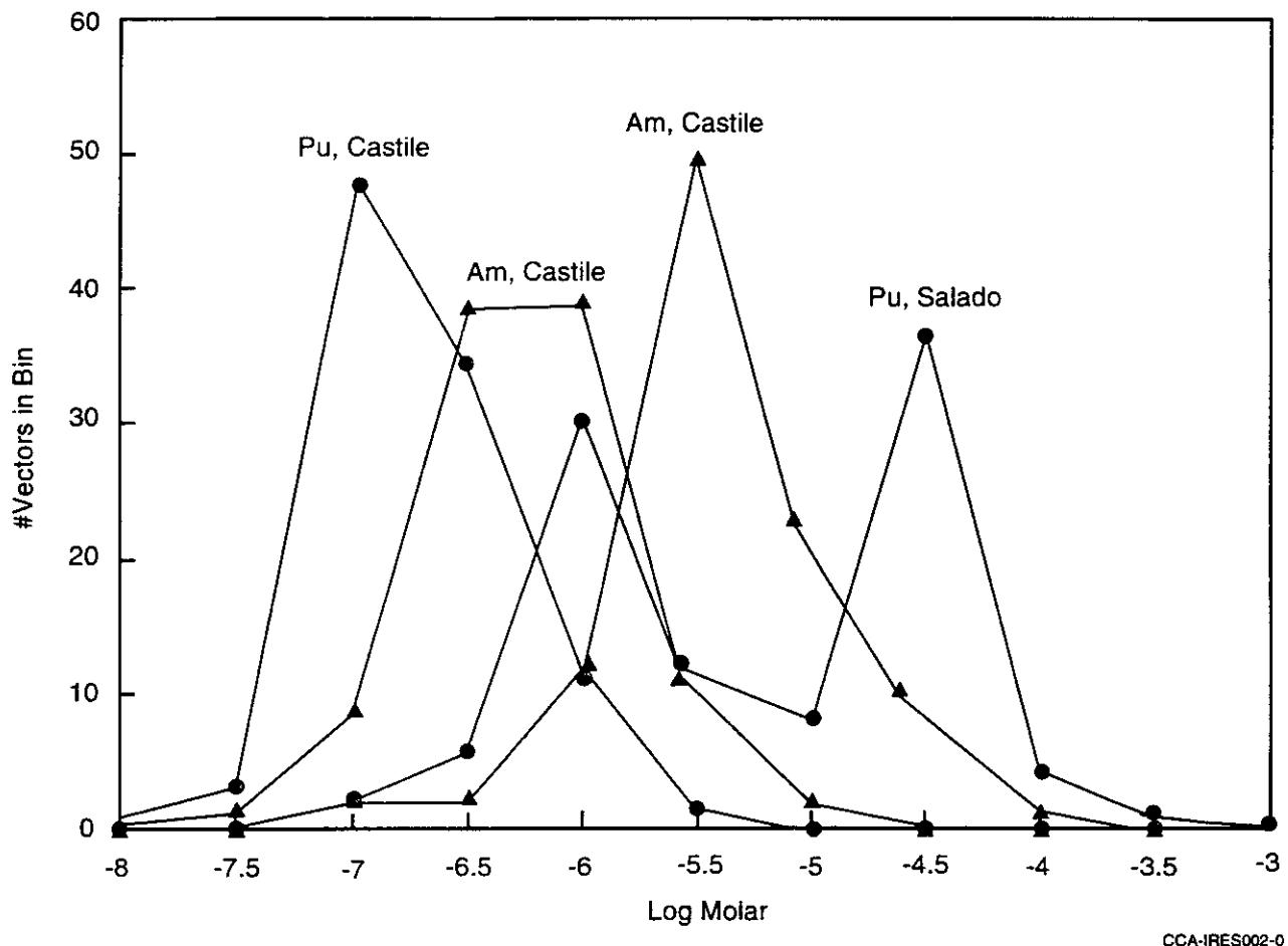
**Figure IRES-2. Total Maximum Concentration (Dissolved and Colloidal)**
