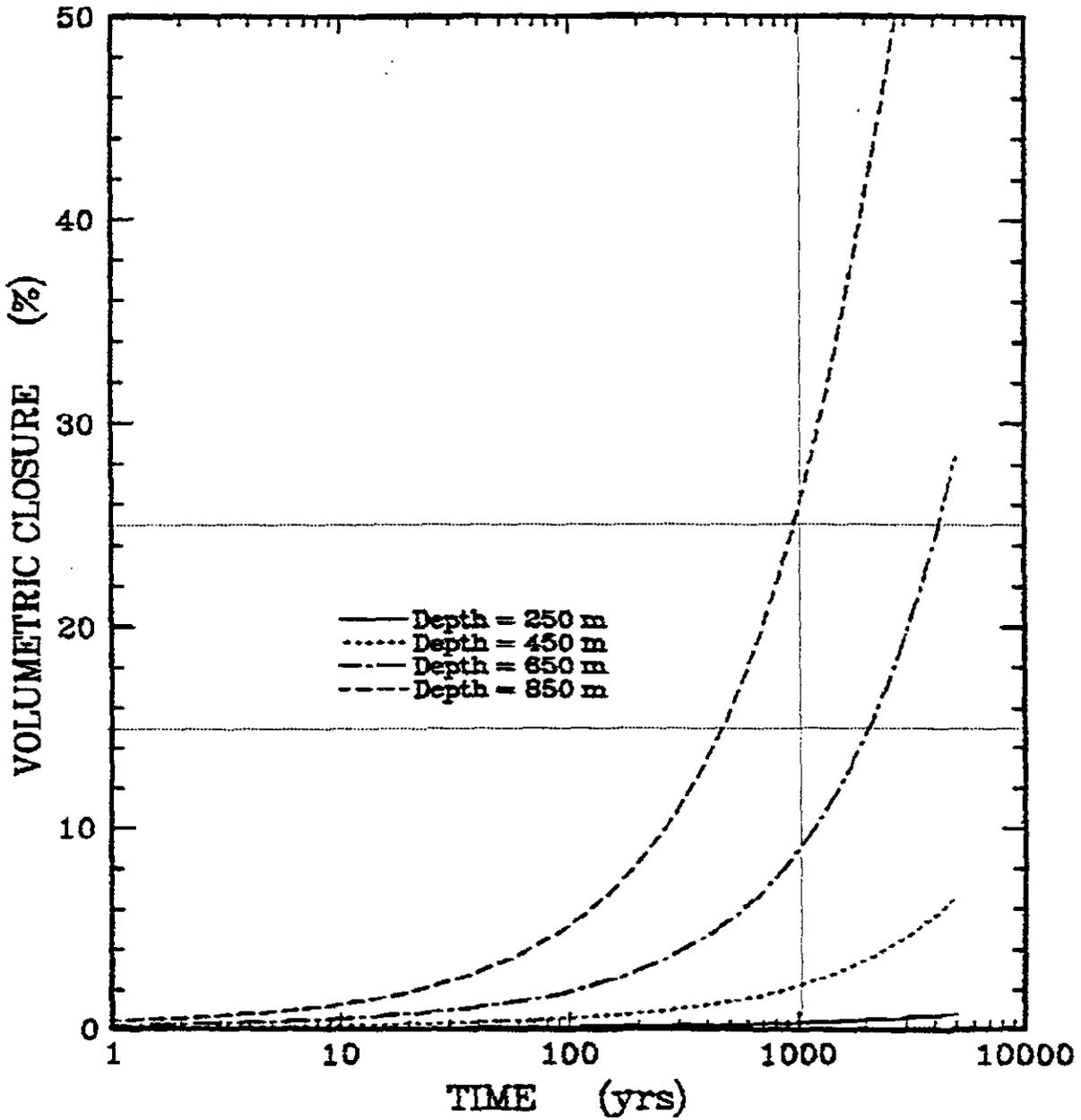
Figure 2. Volumetric Closure as a Function of Time at Four Depths.
