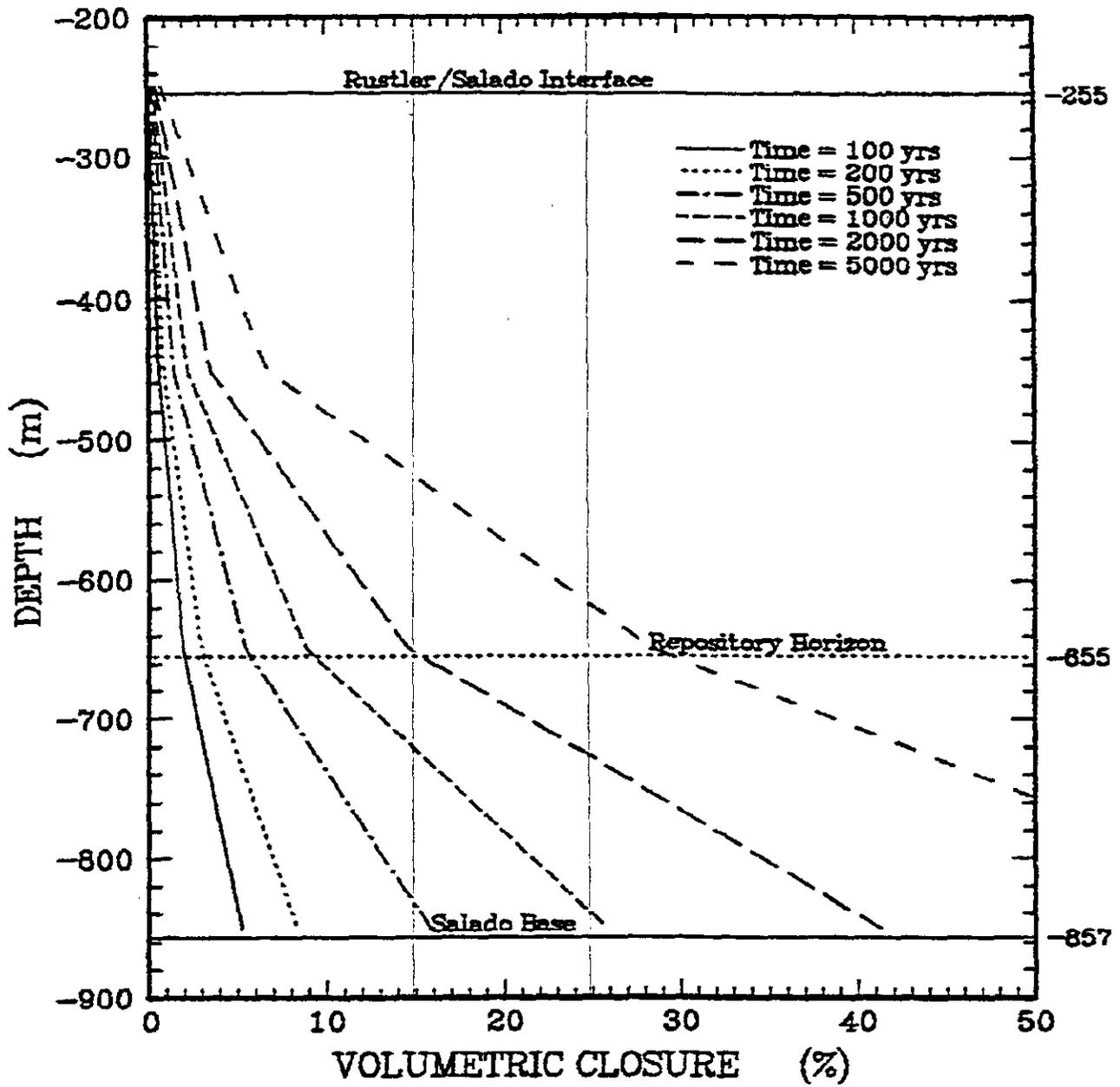
Figure 3. Volumetric Closure as a Function of Depth at Six Representative Times.
