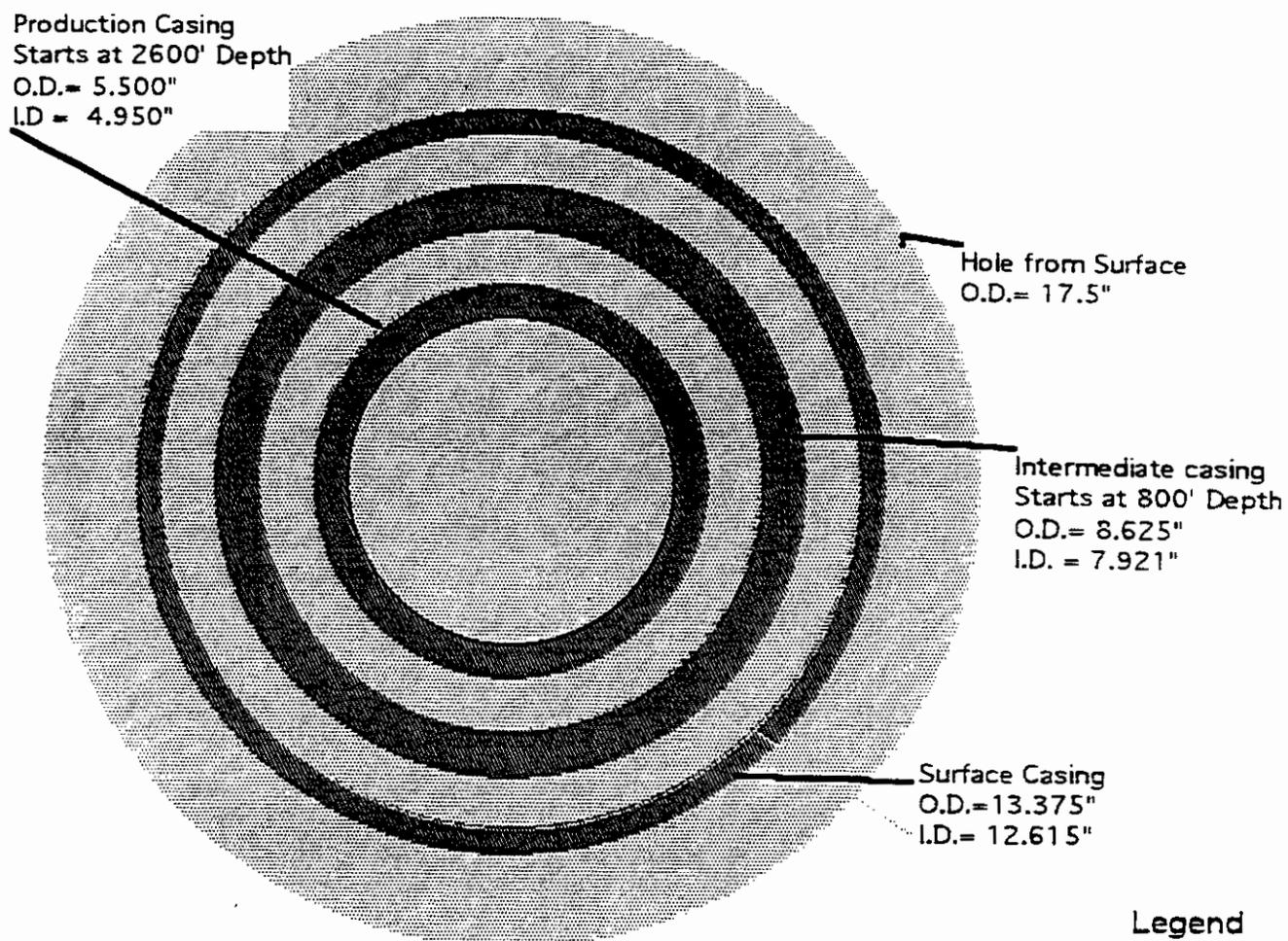
Figure 4: Axial Cross Section of Plugged Borehole
