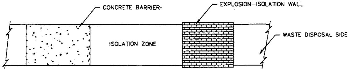
B. CONCRETE BARRIER WITHOUT DRZ REMOVED AND EXPLOSION ISOLATION WALL
