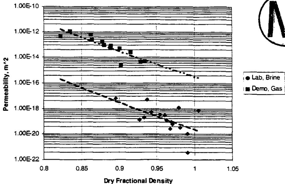
**Figure 4.4.2. Crushed Salt Permeability Data (Same Data as Figure 4.4.1), With Two Power-Law Trend Lines Representing Brine Permeabilities on Lab-Prepared Samples and Gas Permeabilities on Field Demonstration Samples**
