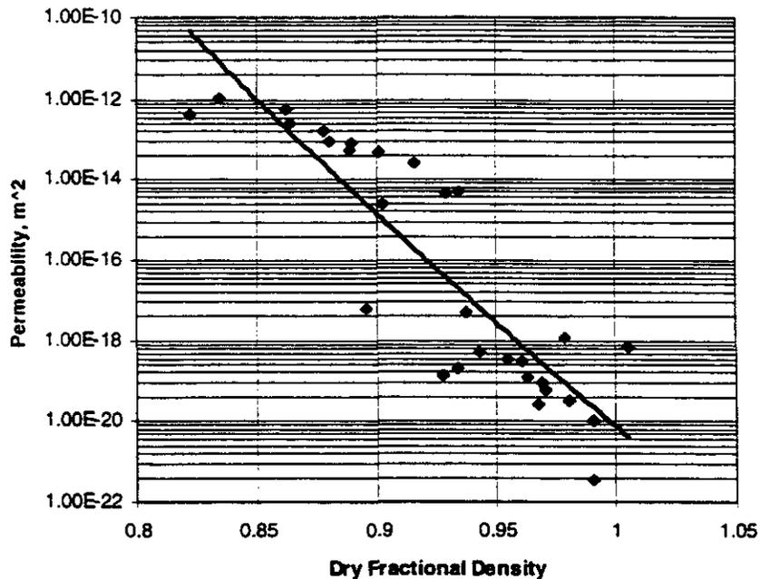
**Figure 4.4.1. Crushed Salt Permeability Data, With Single Power-Law Trend Line**
