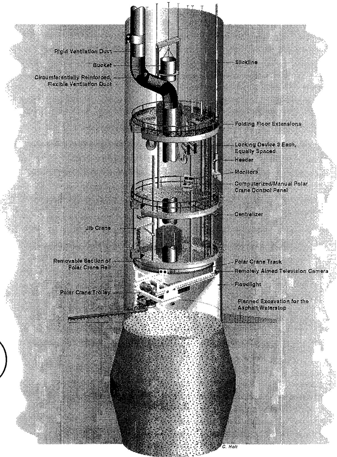
Figure B-2. Multi-deck stage illustrating excavation for asphalt waterstop.
