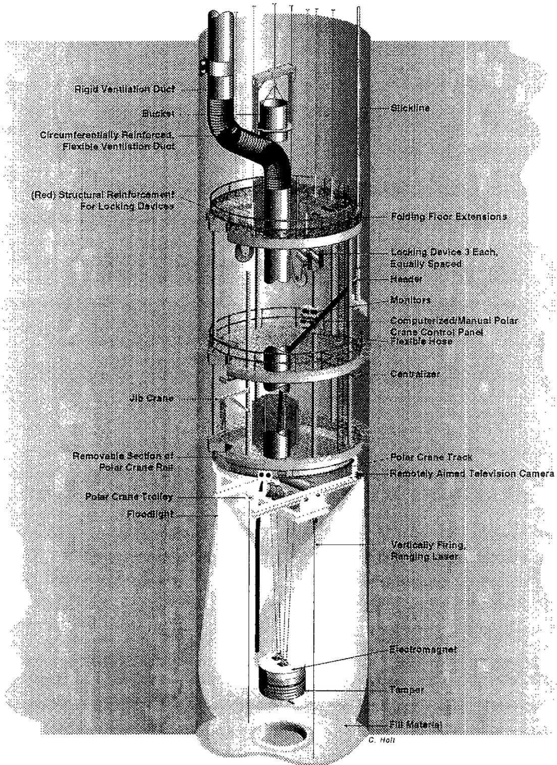
Figure B-1. Multi-deck stage illustrating dynamic compaction.
