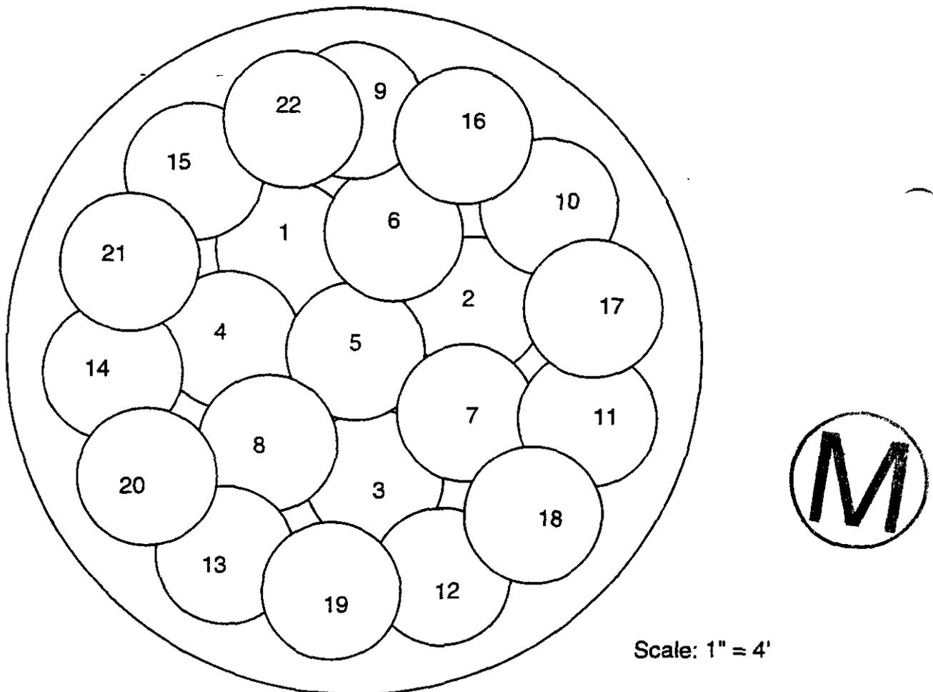
Figure B-4. Drop pattern for 6-m-diameter shaft using a 1.2-m-diameter tamper.
