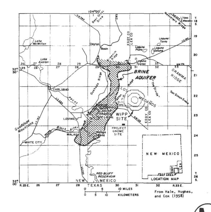
Figure 14.--Approximate areal extent of the "brine aquifer" near the proposed Waste Isolation Pilot Plant (WIPP) site.
