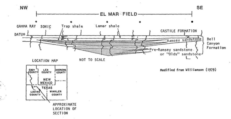
Figure 8.--Generalized geologic section across the El Mar Field, Loving County, Texas.
