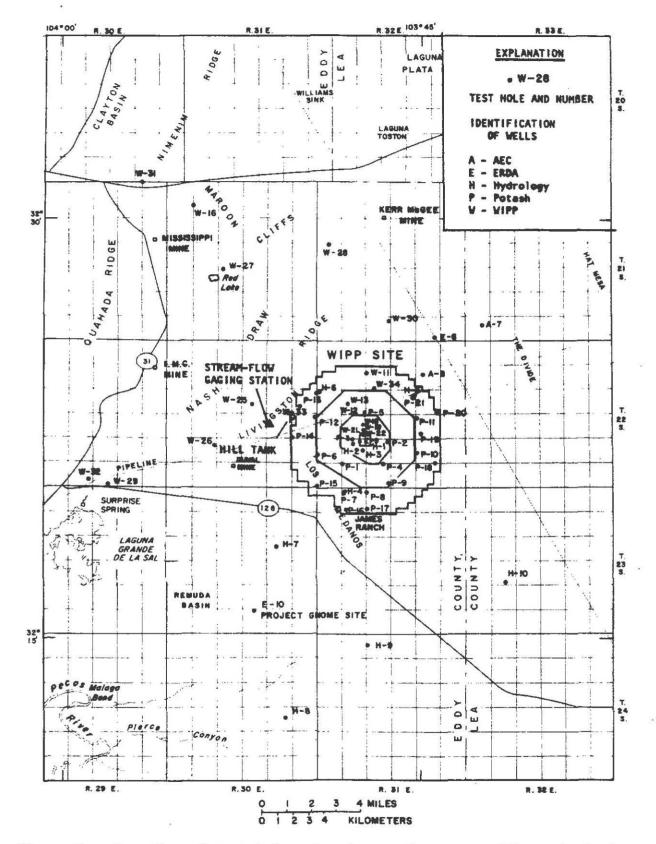
Figure 1a.--Location of test holes at and near the proposed Waste Isolation Pilot Plant (WIPP) site.
