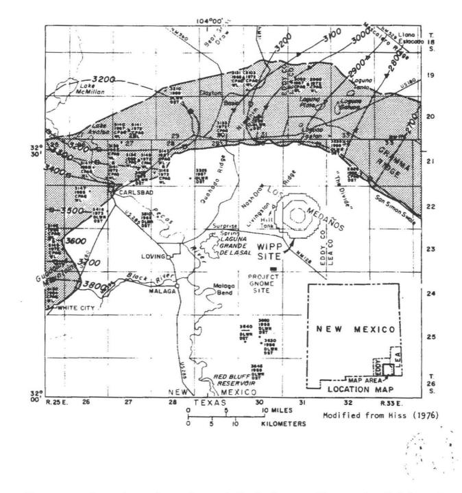
Figure 11.--Potentiometric surface of the Capitan aquifer in the vicinity of the proposed Waste Isolation Pilot Plant (WIPP) site.
