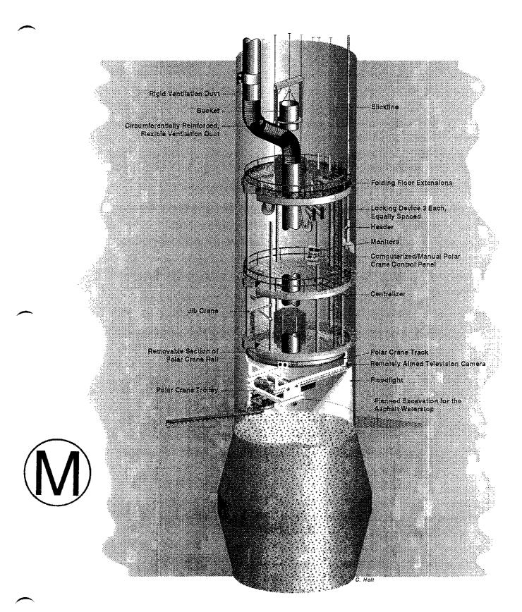
Figure B-2. Multi-deck stage illustrating excavation for asphalt waterstop.
