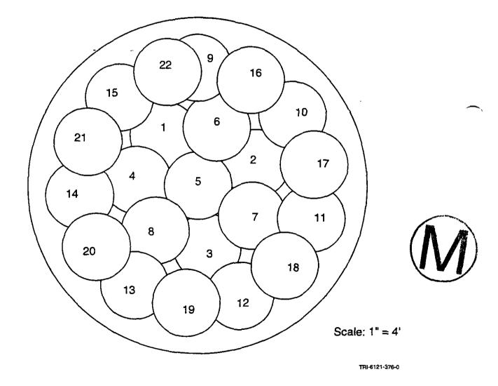
Figure B-4. Drop pattern for 6-m-diameter shaft using a 1.2-m-diameter tamper.
