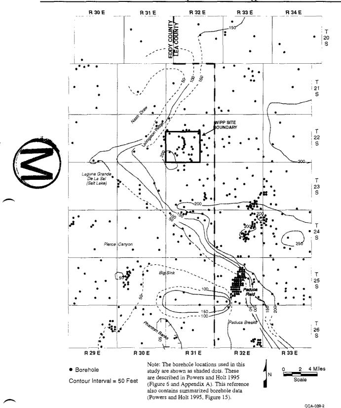
Figure 2-23. Isopach from the Base of MB103 to the Top of the Salado
