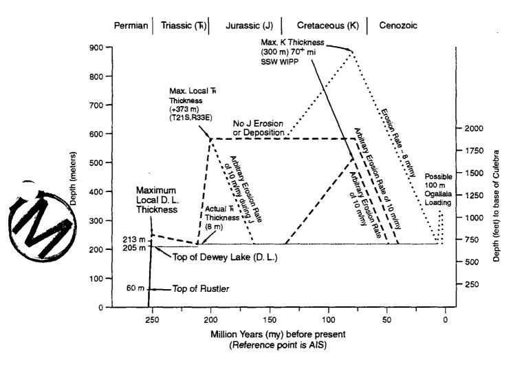
Note: The estimates are made with a reference point and depth to the base of the Culebra at the AIS. Source: Powers and Holt 1995, Figure 34.
