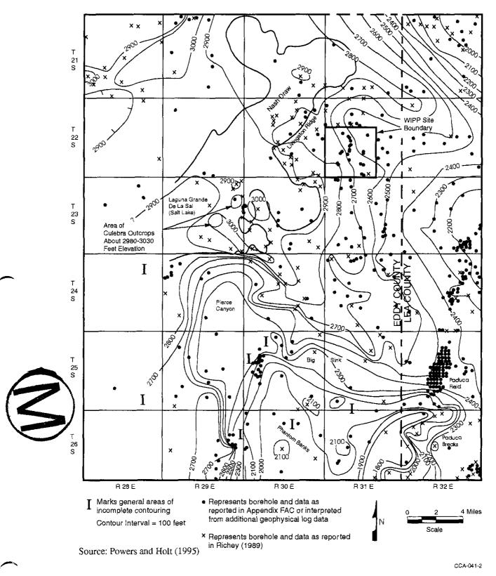
Figure 2-24. Structure Contour Map of Culebra Dolomite Base
