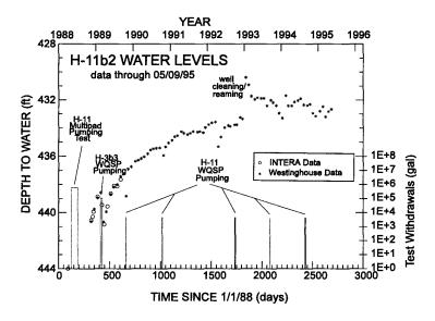
Figure 2.3-8. Well H-11b2 water levels.
