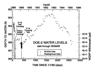
Figure 2.3-22. Well DOE-2 water levels.
