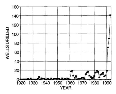
**Figure 2.2-4**. Annual number of oil and gas wells completed in the nine-township area centered on the WIPP Site.
