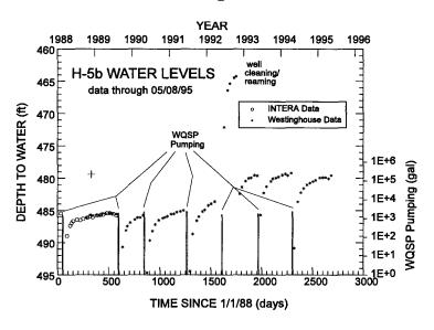
Figure 2.3-21. Well H-5b water levels.
