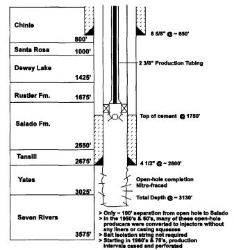
**Figure 2.5.3-7**. Typical Rhodes Yates-Seven Rivers early completion, 1940s-1950s.
