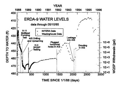
Figure 2.3-17. Well ERDA 9 water levels.
