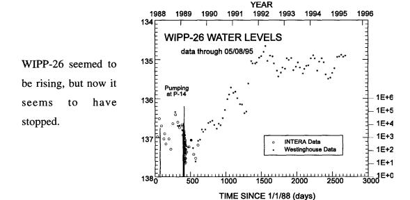
Figure 2.3-27. Well WIPP-26 water levels.
