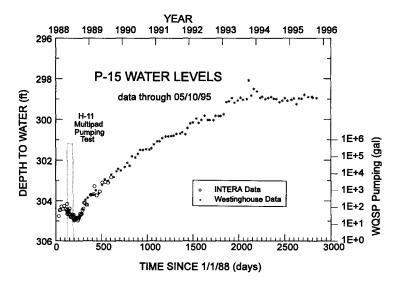
Figure 2.3-9. Well P-15 water levels.
