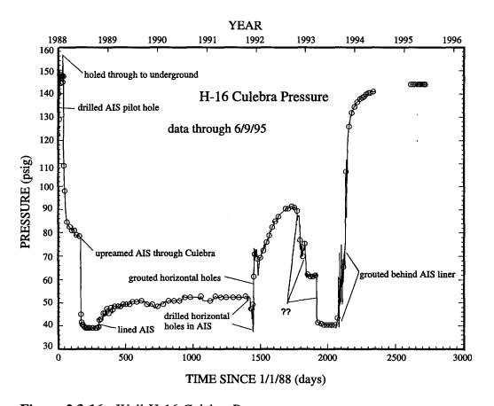
Figure 2.3-16. Well H-16 Culebra Pressures.
