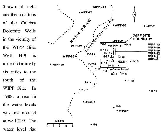
**Figure 2.3-1**. Locations of Culebra Dolomite Wells in the vicinity of the WIPP Site.
