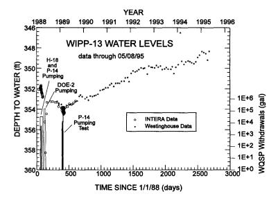
Figure 2.3-23. Well WIPP-13 water levels.
