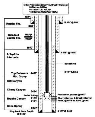
**Figure 2.5.3-5**. Typical Livingston Ridge/Lost Tank Completion.
