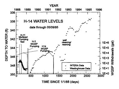
At H-14, there is the same type of response as observed at the other wells - a well cleaning exercise - pumped out - changes in fluid density.
