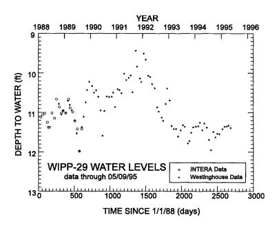
Figure 2.3-29. WIPP-29 water levels.
