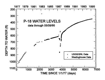
Figure 2.3-31. Well P-18 water levels.
