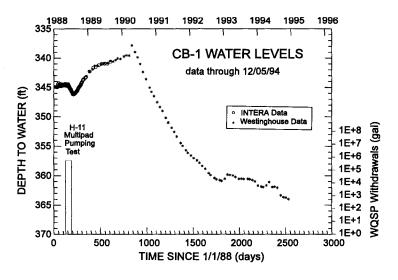
Figure 2.3-6. Well CB-1 water levels.
