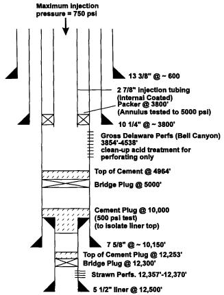
**Figure 2.5.3-9**. Current Salt Water Disposal Well Livingston Ridge Federal #9. Intent filed September 24, 1992.
