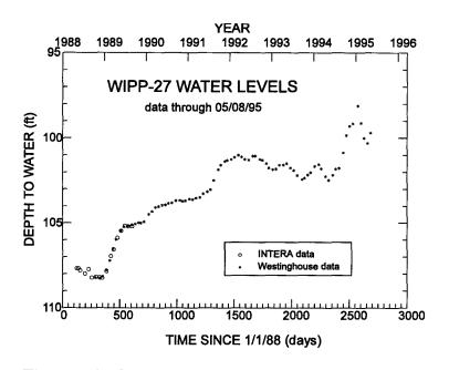
Figure 2.3-28. WIPP-27 water levels.
