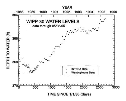
Figure 2.3-30. WIPP-30 water levels.
