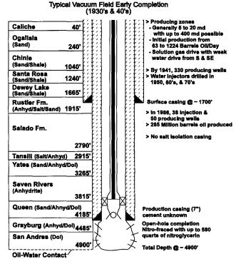
**Figure 2.5.3-6**. Typical Vacuum Field Completion for 1930s and 1940s.
