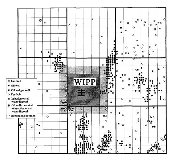
Figure 2.2-2. Oil, gas, and injection wells at WIPP Site, one-mile additional study area, and nine-township project study area.
