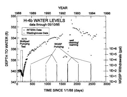
Figure 2.3-7. Well H-4b water levels.
