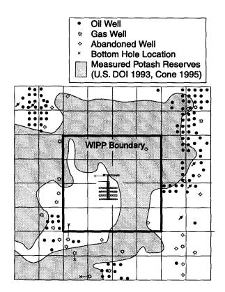
Figure 3-20. Actual oil, gas and injection well boreholes.
