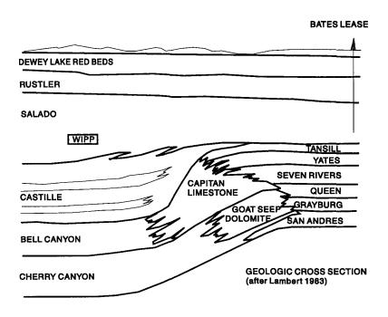
Figure 2.7-1. Geologic cross section at WIPP and Bates Lease (After Lambert 1983).
