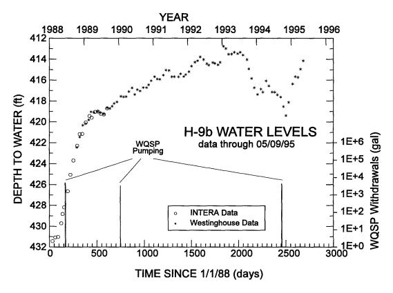
Figure 2.3-2. Well H-9b water levels.
