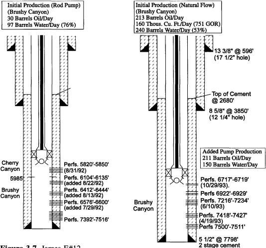
**Figure 3-7**. James E#12. Typical Cabin Lake Completion. After Dan Stoelzel.
