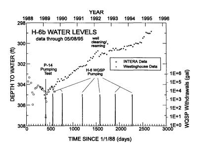
Figure 2.3-24. Well H-6b water levels.
