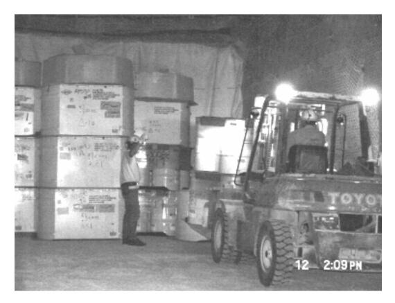
Figure 3. Waste being emplaced in Panel 1. Note stacks of three containers with MgO on top of each stack.
