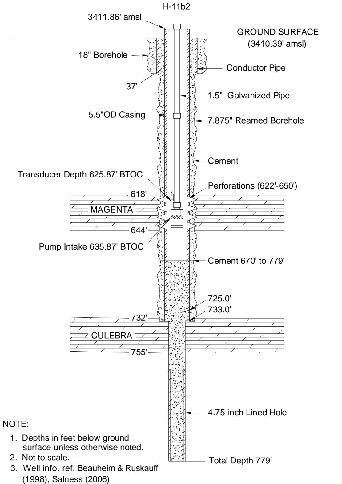
Figure 35. Configuration of well H-11b2 during testing.
