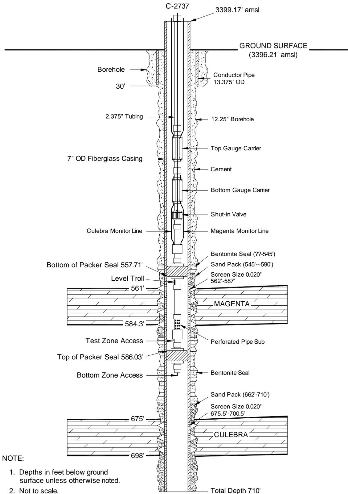
**Figure 25. Configuration of well C-2737 during testing.**
