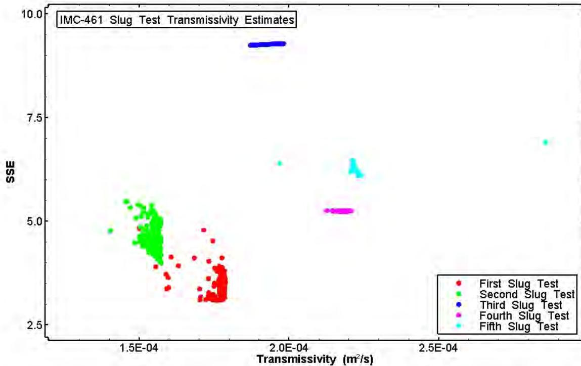
**Figure 14. Formation transmissivity comparison from IMC-461 slug tests.**
