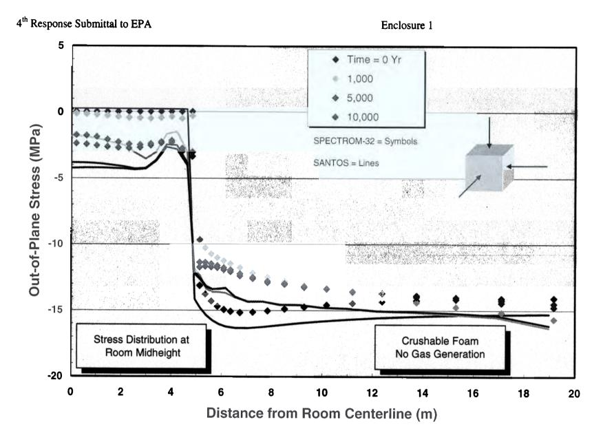
Figure 5. Comparison of SANTOS and SPECTROM-32 Out-of-Plane Stress Results for a TRU Waste Reduced Deviatoric Envelope and No Gas Generation.
