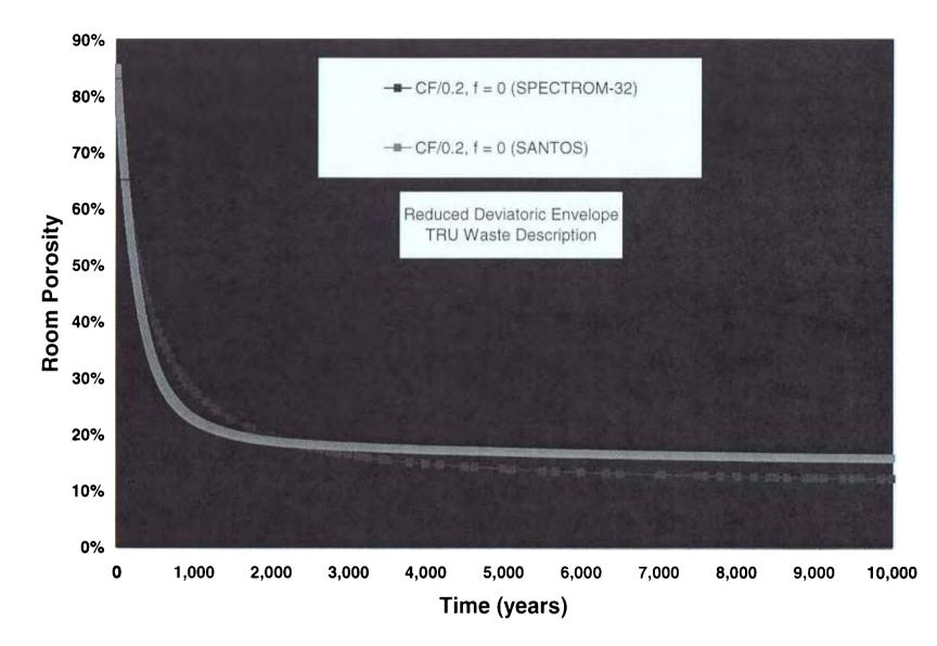
Figure 2. Comparison of SANTOS and SPECTROM-32 Room Porosity Results for a TRU Waste Reduced Deviatoric Envelope and No Gas Generation.
