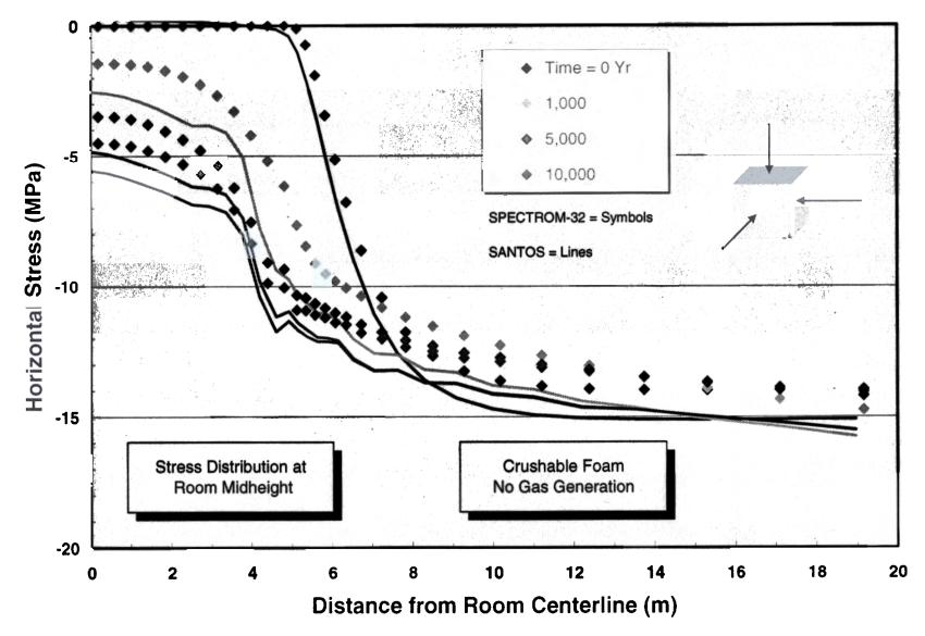
Figure 3. Comparison of SANTOS and SPECTROM-32 Horizontal Stress Results for a TRU Waste Reduced Deviatoric Envelope and No Gas Generation.
