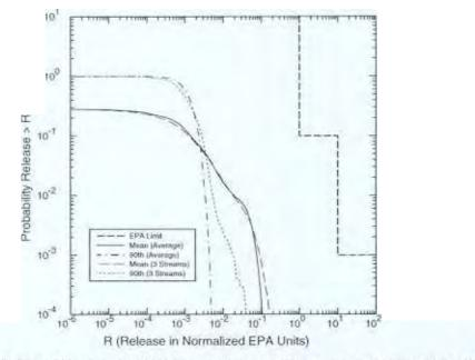
Figure 3. Sensitivity of Spallings Releases to Assumptions About Container-Scale Variability
