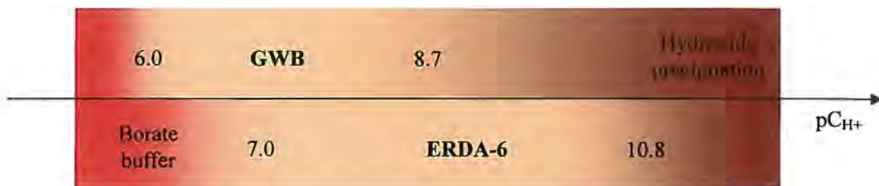
Figure 4-3: Chemical stability of GWB and ERDA-6 brines versus pC_{H^+} . The lower pC_{H^+} value is defined by the buffering capacity and range of borate in the brines. The higher pC_{H^+} value corresponds to the “cloud” point when precipitation occurs. The pC_{H^+} boundaries have an accuracy of \pm 0.5 pH unit.
