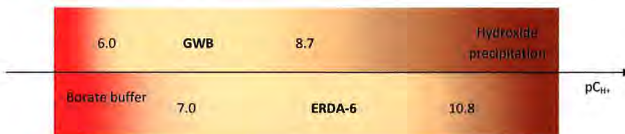
Figure 2. Chemical stability of GWB and ERDA-6 brines versus pC_{H+} [Borkowski 2009, Lucchini 2010]. The lower pC_{H+} value is defined by the buffering capacity and range of borate in the brines. The higher pC_{H+} value corresponds to the “cloud” point when precipitation occurs. The pC_{H+} boundaries have an accuracy of \pm 0.5 pH units.
