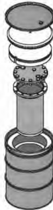
B. Pipe Overpack within a 55-Gallon Drum
