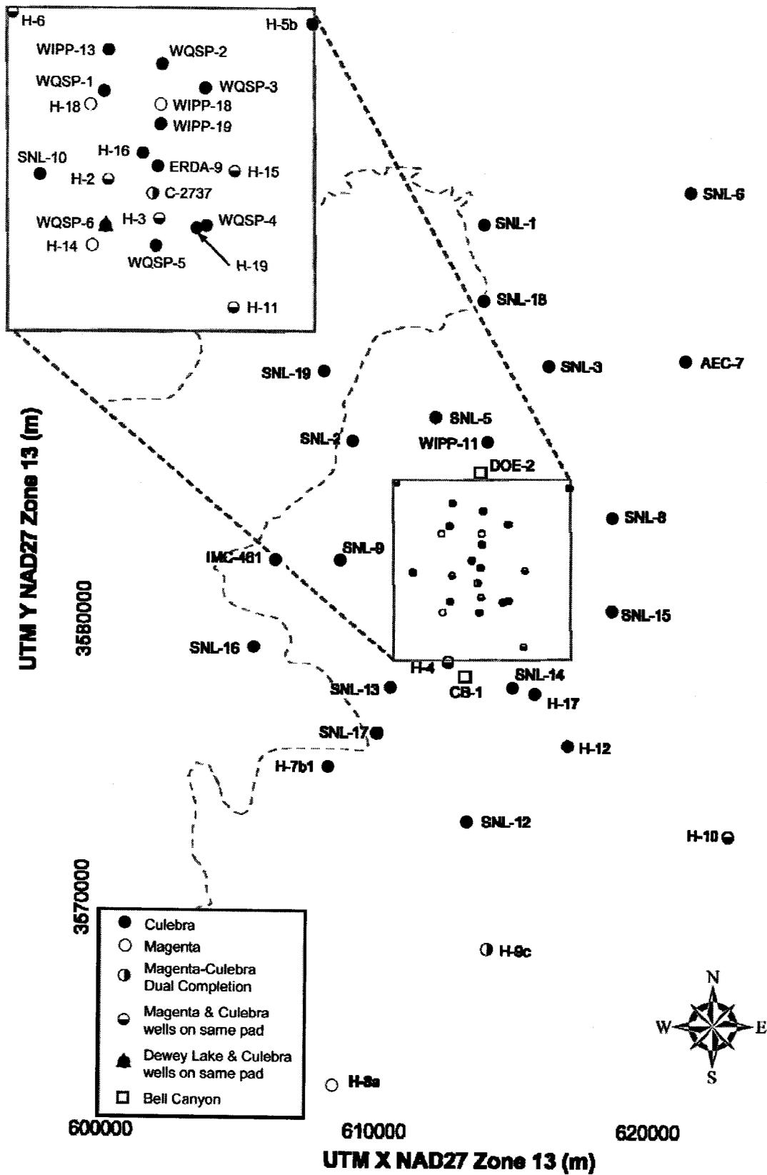
Figure 4-2. The WIPP groundwater monitoring network
