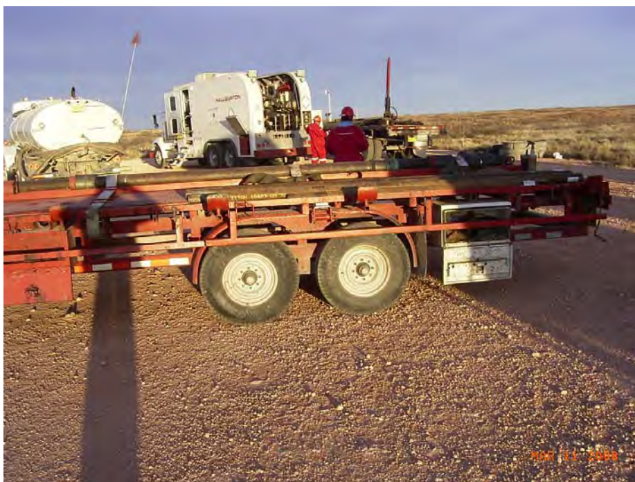
Figure 4 - The Halliburton Logging Truck and Casing Perforating Guns on the Trailer in the Foreground
