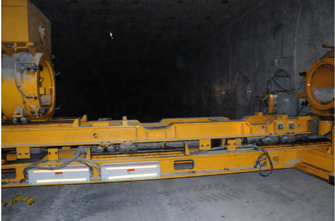
Figure 4 Equipment prepared for RH waste emplacement in Room 7 of Panel 6
