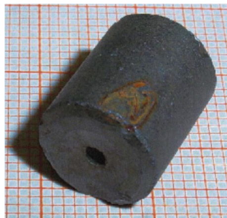
Figure 2. Fuel pellet described by Wallenius et al. 11 where physical dimensions were a key nuclear forensic signature. Reprinted with permission from ref 11. Copyright 2006 Elsevier.
